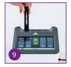
Insert the test strip into the provided cartridge. Place the cartridge containing the test strip into a reader port.
