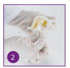
Weigh in 10 g of adequately ground, representative sample into one side of a Whirl-Pak® filter bag. Add one extraction buffer bag into the same side.
