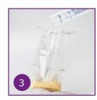
Add 50 ml of distilled, deionized or bottled water to the Whirl-Pak® filter bag.
