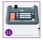
The AgraVision™ Pro detects the test strip via the data matrix code on the strip. Enter sample ID, matrix type and quantitation range.
