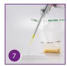
Transfer 100 µl of sample extract supernatant from the filter bag to the microcentrifuge tube (1:11 dilution).\*
