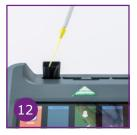
Pipette the sample extract into the cartridge. The reader automatically starts the assay and displays the result when finished.
