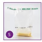
Let the sample settle for 1 minute. ONLY FOR T-2/HT-2: Centrifuge the sample supernatant for 30 seconds at 2000 q.
