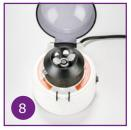
Centrifuge the diluted sample for 30 seconds at 2000 g. (This is the second centrifuge for T-2/HT-2).
