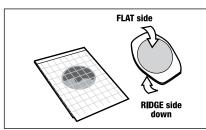
6 With ridge side down, place 3M™ Petrifilm™ Spreader on top film over inoculum.
