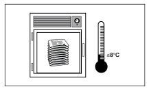
1 Store unopened pouches of plates refrigerated or frozen at temperatures lower than or equal to 8°C (46°F). Use before expiration date on package. Just prior to use, allow unopened pouches to come to room temperature before opening.
