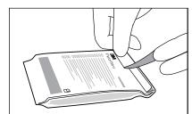
2 Seal by folding the end of the pouch over and applying adhesive tape. To prevent exposure to moisture, do not refrigerate opened pouches. Store resealed pouches in a cool, dry place for no longer than four weeks. Avoid exposure of plates to temperatures >25°C (>77°F) and/or relative humidity >50%.
