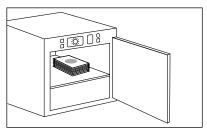
8 Incubate plates with clear side up in stacks of up to 20. It may be necessary to humidify incubator to minimize moisture loss. Please refer to the product instructions for third party validated methods.
